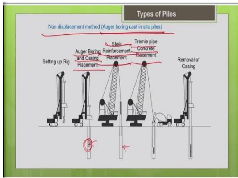
First let us discuss in detail about the non-displacement method. So, the commonly adopted mechanism or a methodology is the auger boring we are going to discuss about this in this lecture. This picture clearly shows you how the auger boring is done. First you set up the rig, then you can say this is the auger bore, it has a spiral or the helical the drilling bit at the bottom which can be rotated by the motor and it is usually accompanied by a casing.
