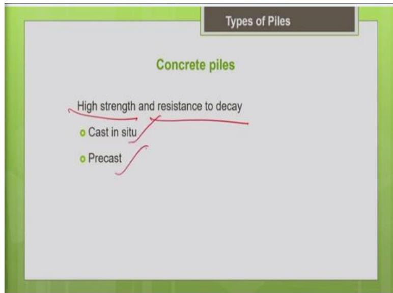
So, the next is about the concrete piles. Obviously, when it compared to the timber pile, it is load bearing capacity is high, there is a high strength and as good resistance to decay, there is no issues of decay. Now so there are based on the method of fabrication, you can either the casted at your project site or you can make it in the factory. So, accordingly you call it a cast in situ concrete piles or precast concrete piles.
