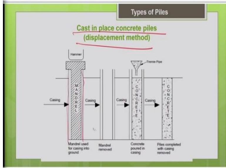
Next is we are going to discuss about the cast in place concrete piles using displacement method. So, first is we are going to drive the steel casing into the ground, steel casing is nothing but the steel pipe, it can be either open at the bottom or it can be closed at the bottom. So, drive the steel casing into the ground this is your casing, you can see that.
