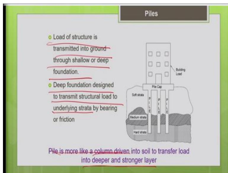
So, as everyone knows, the load of any structure is transferred to the ground to the foundation. So, this foundation can be a shallow foundation or deep foundation. Piles are deep foundation they are examples for deep foundation. So, they are capable of transferring the load from the structure through a weak stratum and it can carry till the depth where a hard bearing stratum is available.
