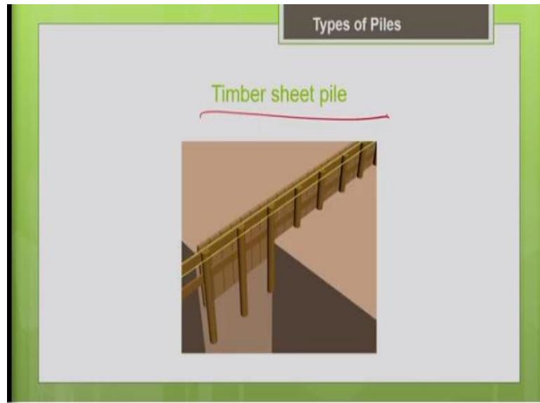
This is the picture of the timber sheet pile, as you know that timber is the oldest material. So, oldest building material we have been using this material for so many centuries, even now we use it wherever the timber is abundant.
