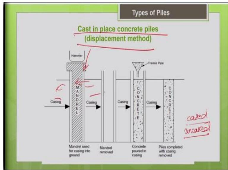
Now how do you drive it with the help of a hammer, you blow the hammer. Since there are chances are the casing may get damaged, and you have to reuse the casing for the further piling. So, that is why commonly you can see that inside the casing they put this mandrel this is the mandrel. So, then you can blow the hammer on the top of the mandrel to avoid the damage to the casing.
