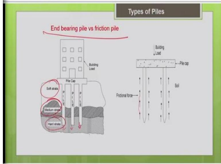
So, other types of applications are end bearing pile and the friction pile, based on the mode of load transfer. So, particularly for the soil with poor bearing capacity and we go for this end bearing pile. So, the end bearing pile has to transfer the load through the weakest strata till it reaches it hard bearing strata which can carry the load. And the load is transferred through the end that is why it is called as the end bearing pile.
